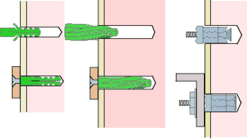
withdraw it so that the top of the plug is in line with the surface. The plug expands to fit the hole tightly as the screw is driven home.
