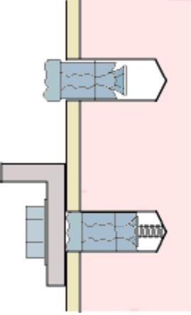
Bolt type inserts incorporate a thread in the cone and a bolt is inserted from the wall surface, different lengths of bolt are available for workpieces of different thicknesses. The hole in the wall needs to be deep enough to ensure that the bolt does not bottom when it is fully tightened.
