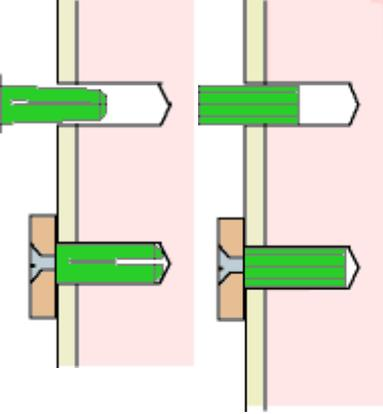
Lightweight blocks can be drilled very easily using a hand-brace or a power drill without hammer action. A risk with these blocks is that they are not very 'forgiving', a small amount of pressure in the wrong direction and the drill bit will be away where you never intended it to go.
